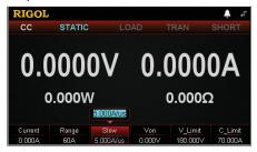
Current slew rate is defined as the rate at which the two set currents switch from one setting to another. The range of the current slew rate is from 0.001 A/us to 5 A/us.
