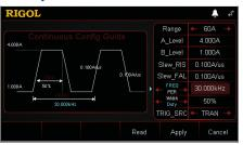
Transient test function enables the load to periodically switch between two set currents (Level A and Level B). The highest transient frequency in CC mode can reach up to 30 kHz
